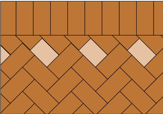
Alternative recommendation – insertion of pavers cut to three quarter length.
