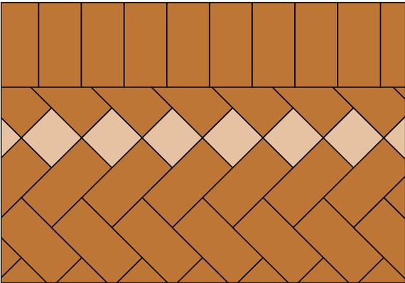
Recommended insertion of pavers cut to half length.
